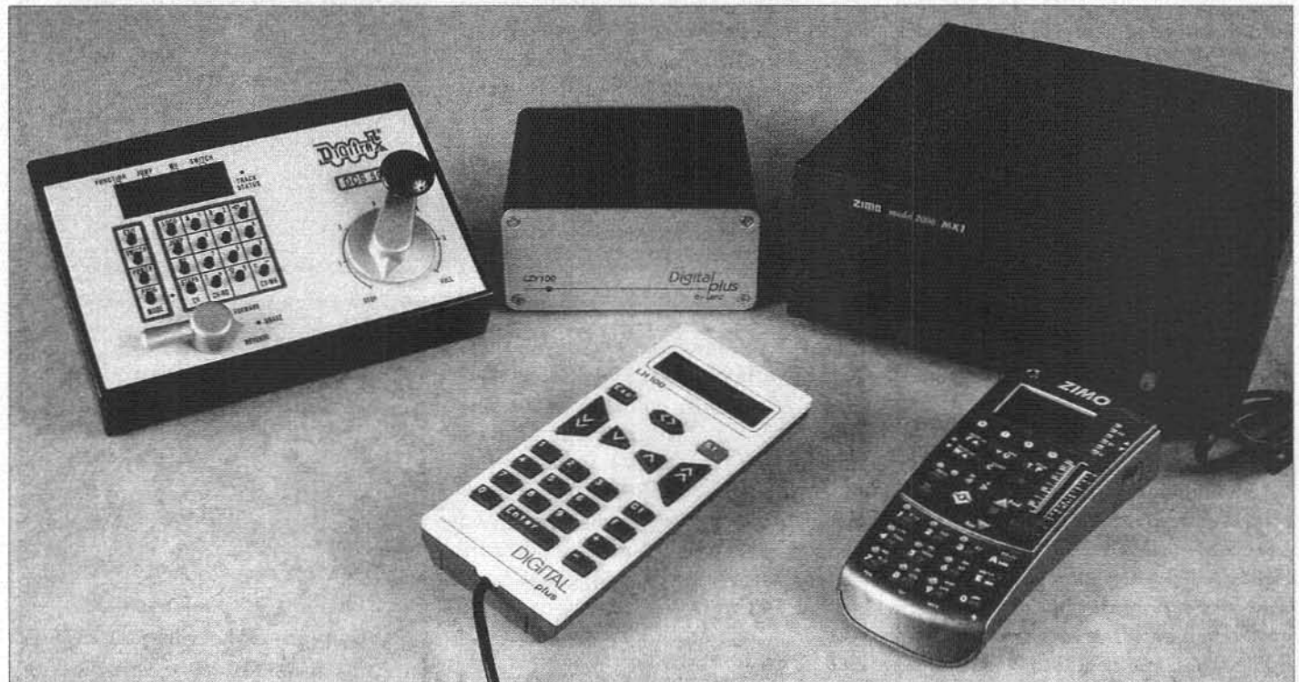
Project DCC will be exploring the use of three different DCC systems. Shown on the left is the Digitrax Zephyr, in the middle the Lenz Set-100, and on the right the
